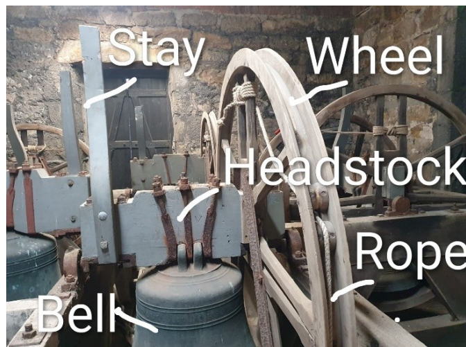
The parts of a church bell (Rick Keeves)
